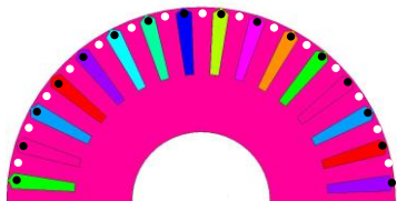
Fig. 1. Sample elements in rotor teeth and bars over one pole pair pitch
